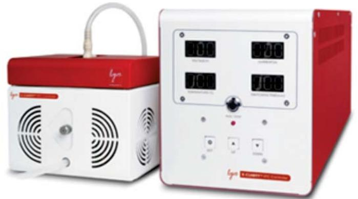
The X-CLARITY<sup>™</sup> ETC Controller works as both a power supply and a temperature controller. The tissue sample is placed inside the X-CLARITY<sup>™</sup> ETC Chamber where it undergoes electrophoresis to remove lipids. Clearing buffer is continually circulated through the chamber under temperature controlled conditions, minimizing the probability of artifacts arising due to poor temperature control.
